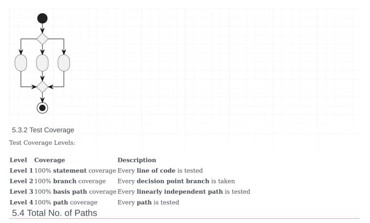
Total No. of Paths *P* tested in **Level 4**: 100% **path** coverage testing:
